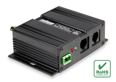
Using the 12-84 Relay Receiver, devices can be controlled remotely by sending commands from a portable or fixed location paging transmitter or wide area paging network to switch relays on or off. It is available in two versions, a VHF 12-84-7150 and a UHF 12-84-7450.
