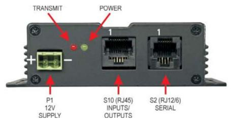
Pin numbering: looking into the sockets with the power connector on the left, pin 1 is on the left.
